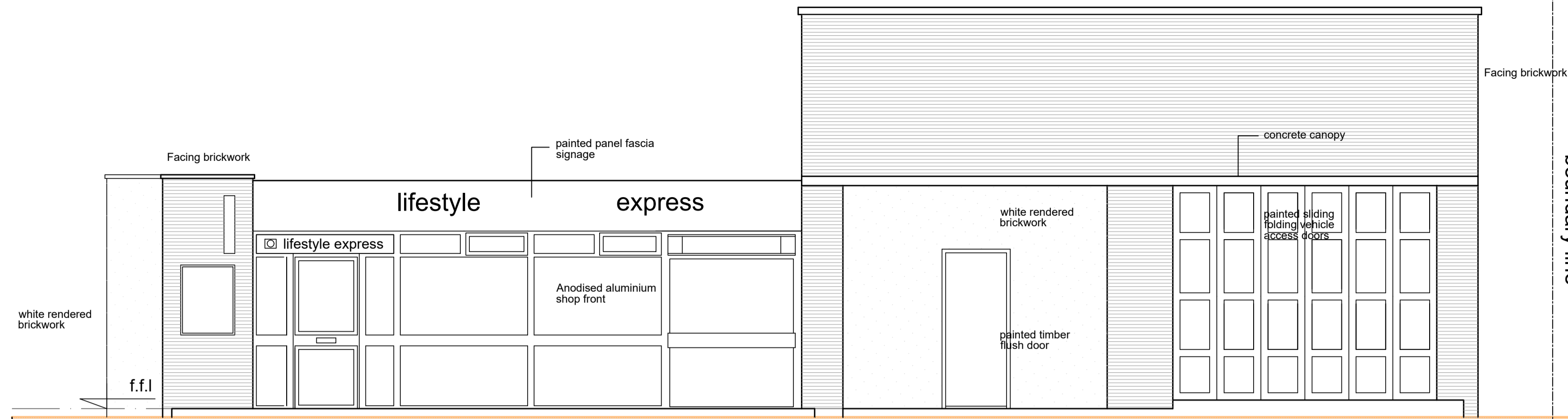
Existing front south facing elevation
